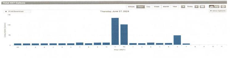
Normal water usage after all leaks fixed. Graph shows hourly flows ranging from 2 gal/hr to 45 gal/hr. Graph shows 50% of the day there was zero usage. No presence of a leak.
